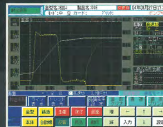
Shot profiles and machine motions can be displayed; alarms and their output methods can be set.
