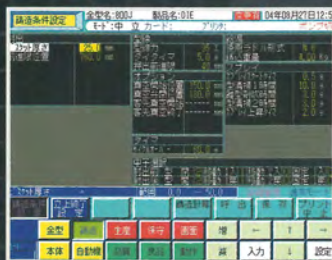
Various conditions for casting can be set, and the batch loading is possible.
