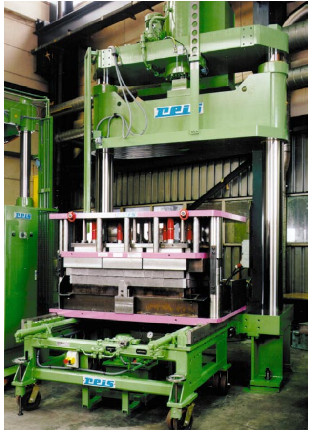
Trim presses with hydraulic tool change slides for large, heavy tools. Change-over via pushing a button, easy and quick.
