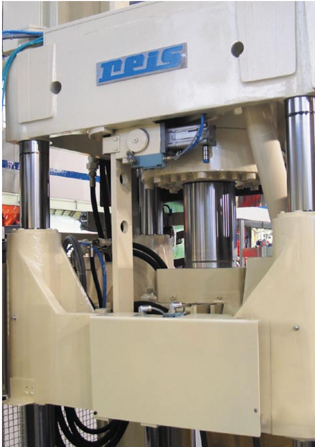
Mechanics suitable for foundries with extremely low-maintenance and low-play 3-or 4-column guidings.
