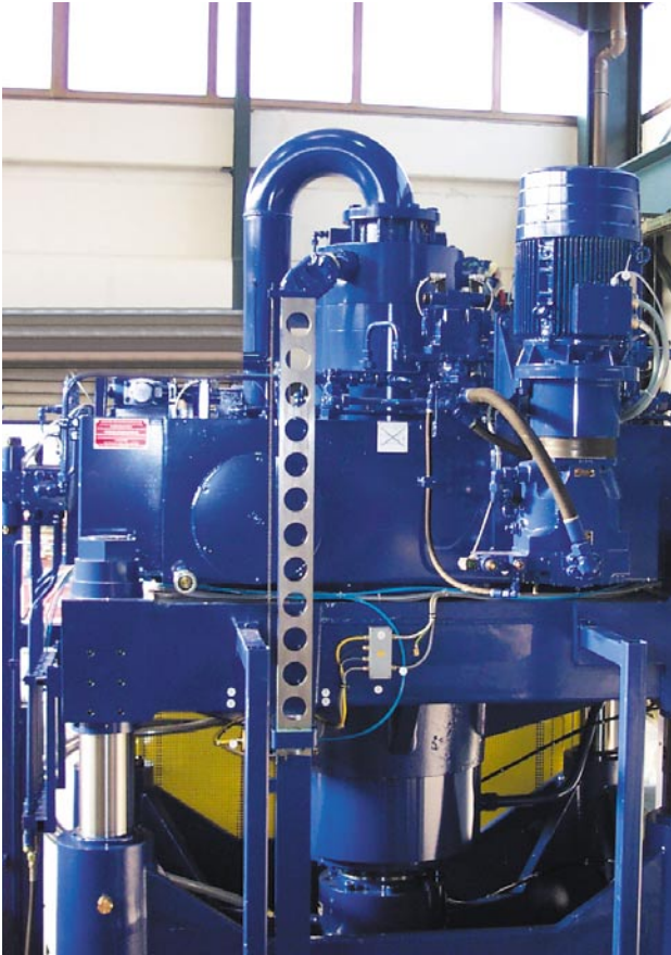
Hydraulic unit at a hydraulic high capacity press, easy-to-service, reliable.
