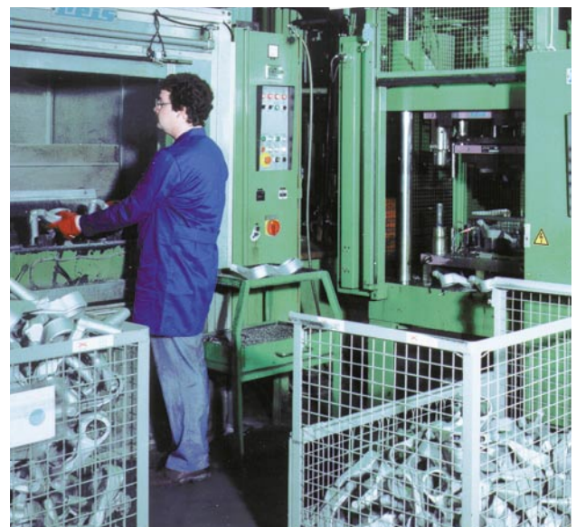
Complete trimming of aluminum sand parts. Manual operation in combination with a separate REIS saw.
