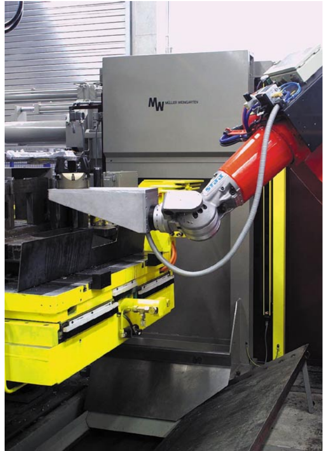
Free loading of a press by means of robot in an automatic casting cell.
