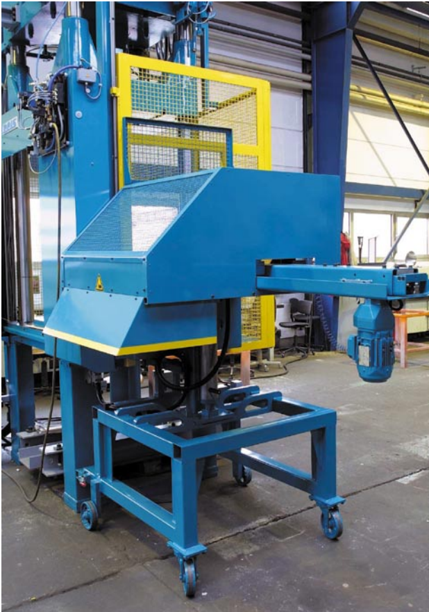
Part removal for output and separation of finished parts. Adjustable in height, easy to handle. Movable for tool change.
