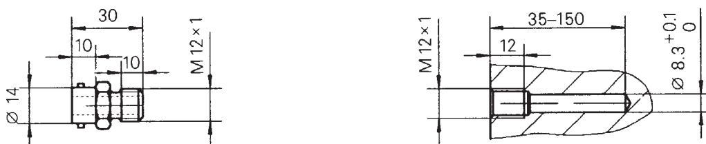
Fig. 4: Bayonet coupling and drilling scheme
